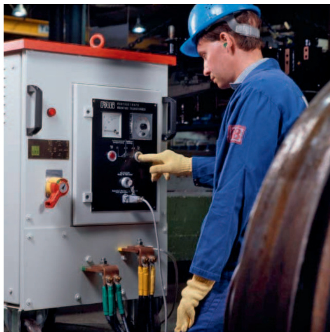
7. The required heating time is set on the time relay. The transformer is started.
