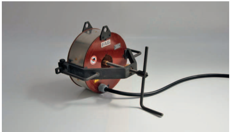
11: Induction coil with withdrawal spindle (on request)
