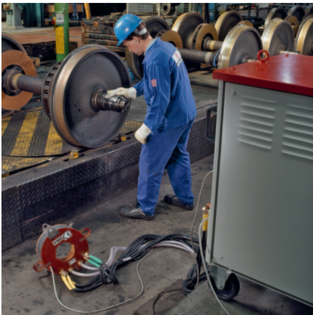
2. The bearing inner rings and adjacent parts are cleaned.
