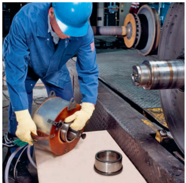
11. The temperature of the inner rings should be checked and, if necessary, the rings should be demagnetised.
