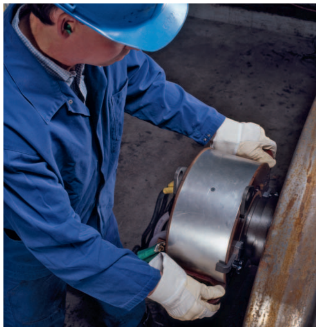
5. The catches on the rear side of the coil are locked.
