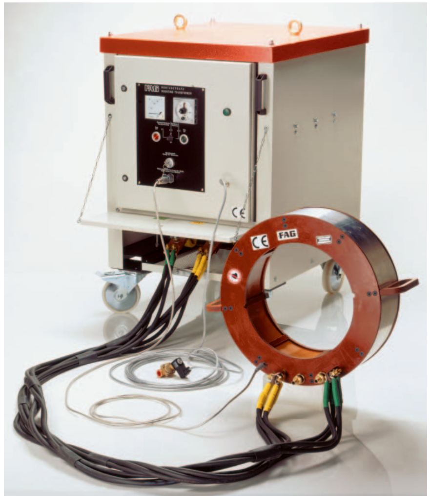
13: FAG induction heating device for low voltage with transformer for dismantling the inner rings of cylindrical roller bearings
