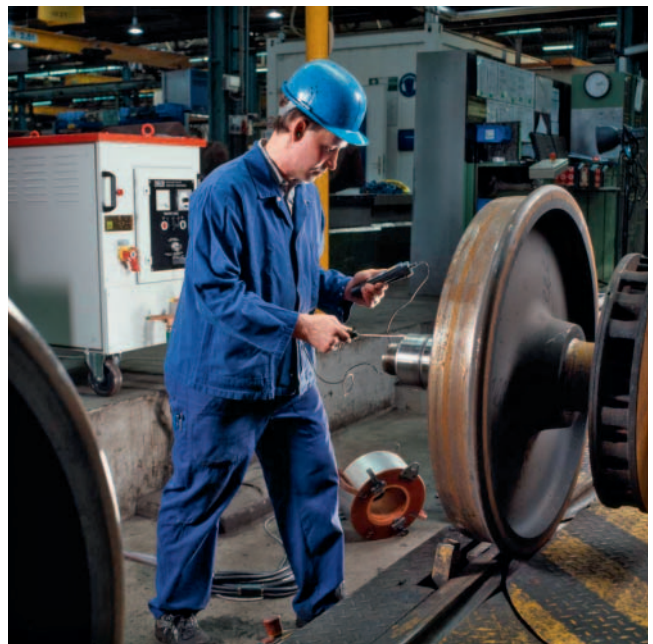
3. The initial temperature of the bearing and shaft journal are monitored using the FAG temperature gauge TEMP-CHECK-CONTACT.
